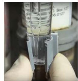
A continuous flow of sample through the tube prevents contamination from atmospheric oxygen. When the operator submerges the vacuum-sealed ampoule in the flowing sample and snaps the tip, sample is drawn into the ampoule. The highly sensitive colorimetric Rhodazine D™ reagent reacts instantaneously to produce a pink color.
