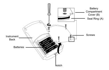
To ensure that the instrument is waterproof:
