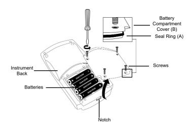
To ensure that the instrument is waterproof:
