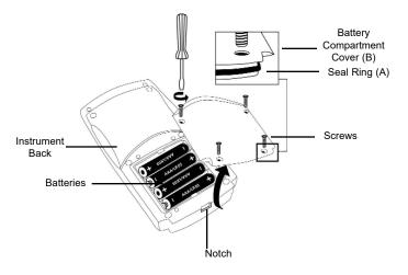
To ensure that the instrument is waterproof:
